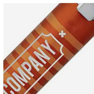
Process identical to screen printing but orientated for printing on circular products, such as ball pens.
