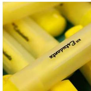
Ideal technique for small objects and curved shapes, as the transfer of ink is made through a silicone pad that adapts to them.
