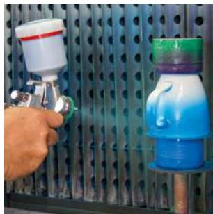
Spraying organic colours on the external surface of white porcelain mugs. After baking, the mug is ready for other printing techniques, such as firing or sandblasting.
