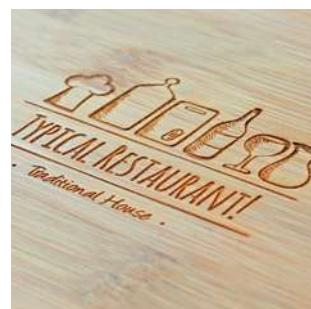
Use of a high-precision laser beam, allowing for low-relief engraving. This laser can be fibre optic, suitable for metals, or CO2, suitable for wood and cork, or UV, suitable for glass.
